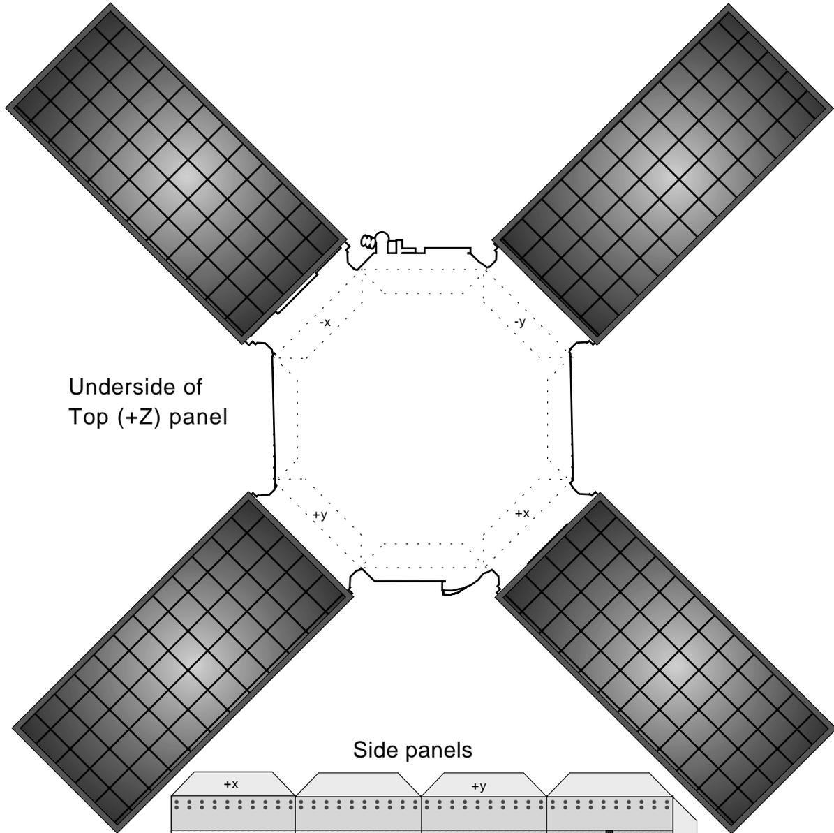
3. Score the lines between side panels, as well as the lines between tabs and panels.
